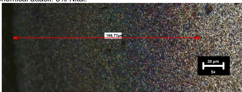
Figure 8. Micrograph of sample 2 (Green Coconut Charcoal media, soaking time of 4 hours) steel. Chemical attack: 3% Nital.
