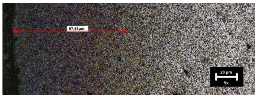
Figure 7. Micrograph of sample 1 (Green Coconut Charcoal media, soaking time of 2 hours) steel. Chemical attack: 3% Nital.
